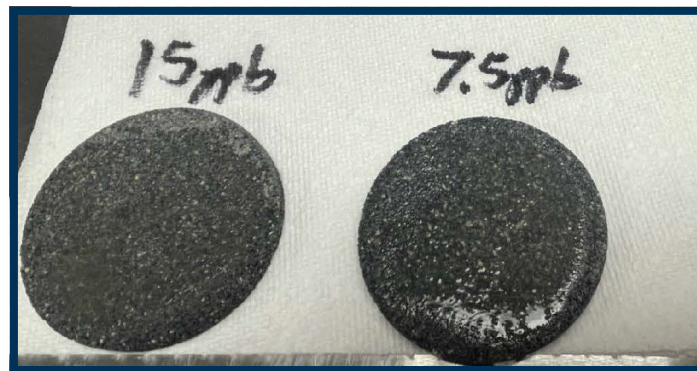
160 micron ceramic disk –(Left to right) 15ppb UFS-LCM100 & 7.5ppb UFS-LCM100 in Bentonite-polymer DF
